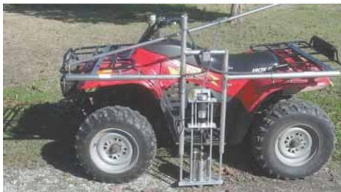
Sampler runs off a 12-volt electric motor and has adjustable depth settings from 4 to 10 in. "You manually control how fast you take the sample," says Mike Machek.
