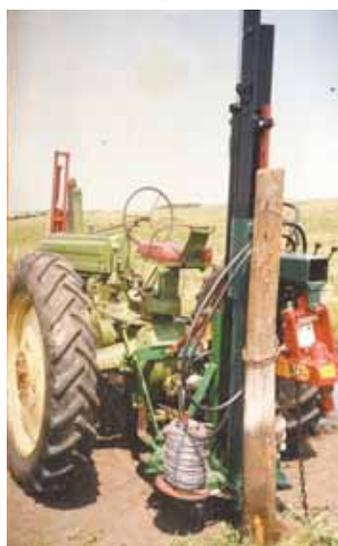
To pull posts out of the ground, Fisher hooks a chain to a sleeve on the mast that holds the auger.
