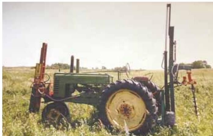
Dennis Fisher uses both ends of his John Deere A tractor to install fence posts. A big Shaver post driver mounts on front and a 4-in. auger operates under pressure on back.
