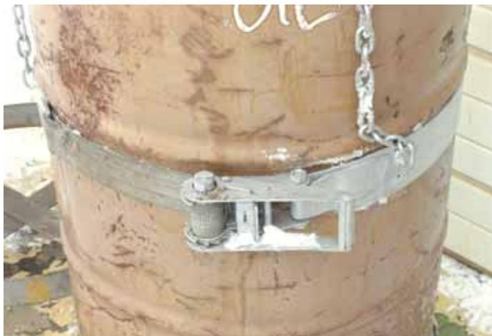
**Vertical drum lifter uses the fuel tank strap from a semi-truck and a "load-securing" ratchet strap to lift drum vertically.**
