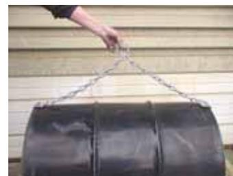
**Horizontal drum lifter consists of a 4-ft. long chain with curved metal brackets welded to each end.**
