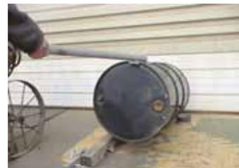
**Operator grabs onto drum laying horizontally and stands it up by hand.**
