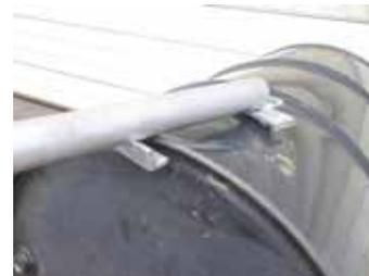
**Drum tipper works like a big prybar and consists of a long pipe with 2 short angle irons spaced about 10 in. apart.**
