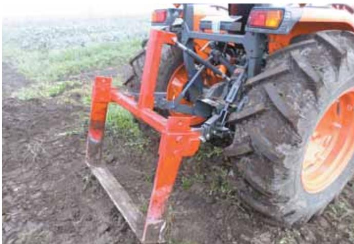
Bed Lifter blade passes under root crops, lifting and breaking up the packed soil to make harvesting easier.
