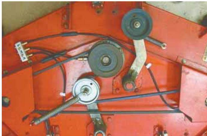
Home-built manifold block distributes grease through individual lines to each grease point on Glander's mower deck.
