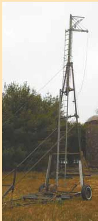
Bill Fluhrer built this hydraulic-operated ladder that reaches up to 35 ft. high. He uses his tractor to pull it around and also to operate the hydraulics.
