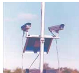
Laser light system mounts on a 15-ft. tall mast and includes 2 lasers that can be adjusted in any direction and up or down.
