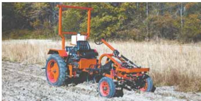
Oggun Tractor has modernized the old Allis Chalmers G tractor with independent hydraulic drive, steering, and lift. "Independent hydraulic drive allows zero-turn capability simply by stepping on one of the brake pedals," says Locky Catron.
