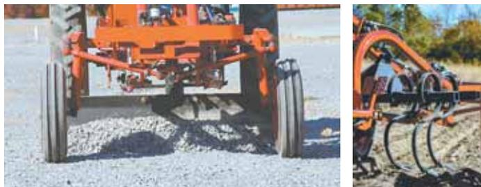
Front and back wheel spacing can be adjusted in 2-in. increments from 36 to 60 in. Tractor's extended frame allows the use of belly-hung implements.
