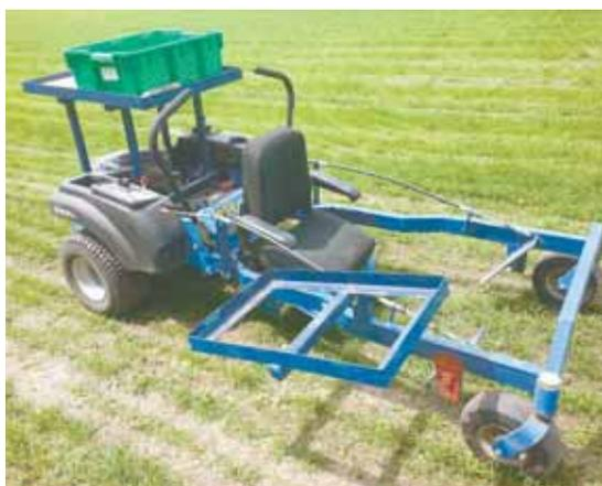
**Holliday converted a Dixon zero-turn riding mower into this asparagus harvester, eliminating the need to bend to pick spears.**
