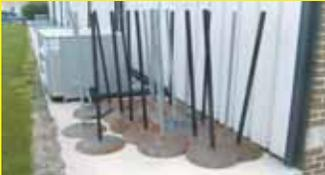
Here's an idea I saw recently to make stanchions to hold yellow caution ribbons or to rope off areas to control crowds. You weld 4-ft. lengths of 1-in. pipe onto disk blades with the concave side faced down. Works great. (Rex Gogerty, Hubbard, Iowa)
