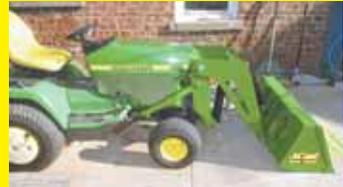
I'm still getting responses from your readers on these two loaders. Now I've come up with yet another loader design for the Deere 445. This loader has a 48-in. wide bucket that lifts 60 in. high and operates off the tractor's standard hydraulic system. Works great for material handling, snow removal and landscape work.
