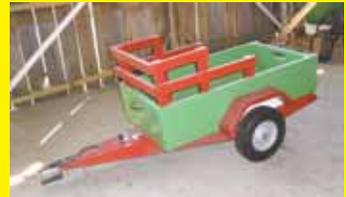
The box measures 24 in. wide by 30 in. long, and the back side is hinged so it can be raised to dump. The tailgate can be pulled out when needed. A spring-loaded catch on front keeps the box from rattling around when it's empty, and a metal foot keeps the trailer's hitch off the ground. (Robert H. Meacham, trainman109@att.net)
