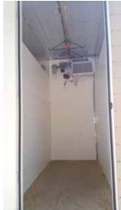
Bob Meyer uses this trailer-mounted cooler to chill wild game taken in warm weather. The insulated box on wheels is fitted with an air conditioner and a CoolBot controller.
