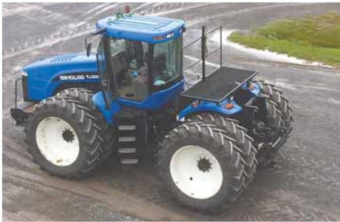
Max Kaiser made a secure platform for pruning trees along field edges by mounting a home-built metal deck on back of his New Holland 4-WD articulated tractor.
