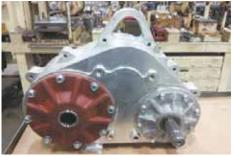
Custom gearbox can be bolted to either side of a combine header auger to replace the belt drive.
