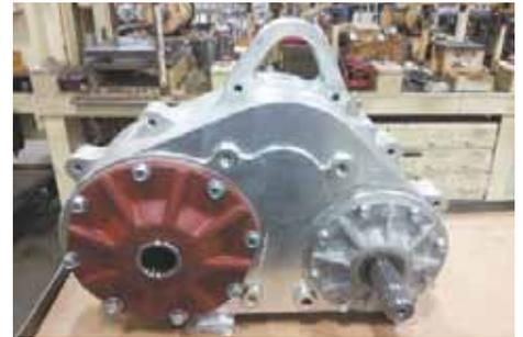
Custom gearbox can be bolted to either side of a combine header auger to replace the belt drive.
