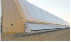
Bunk system attaches to side of building and comes with hinged polymer bins and a roof. Operator pushes a button to open roof and then loads feed into bunk.
