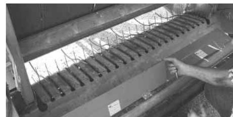
"Leaf Saver" fills a gap to keep hay leaves from falling between baler's rear axle and pickup head.
