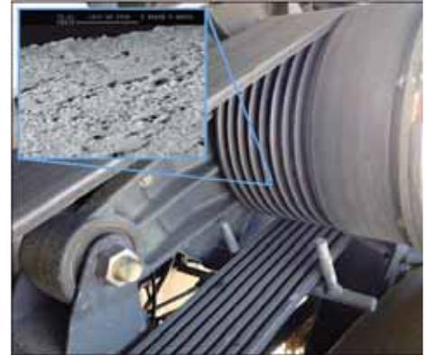
Photo shows pulley treated with Vulcan Grip on a Claas 980 self-propelled forage harvester. Vulcan Grip’s ultra-hard microtexture (inset) resembles an asphalt road surface under a microscope.
