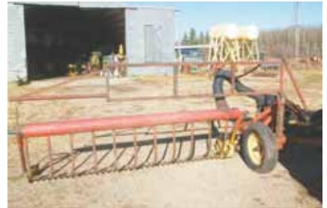
To mount the air reel, he fabricated a support using the boom off an old crop sprayer. "If the boom hits a solid object, it's designed to break away," says Rogers.
