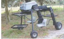
Engine and drivetrain mount 4 ft. off the ground, above operators. Both rear wheels are belt-driven.
