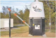
Corn Xpress is a giant vending machine that dispenses fresh corn on demand. An unloading auger feeds into trucks, trailers, or buckets.
