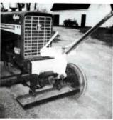
on one end. The front spear's mounting bracket is hinged, allowing the cylinder mounted beneath it to push the bale up to a 45 degree angle. The rear-mounted spear is mounted on a heavy-duty steel framework that attaches to the tractor's 3-pt. The spear is hinged on top of a vertical steel pipe, allowing the spear to raise the bale on end at a 45 degree angle and lift it 4 ft. off the ground when the 3-pt. is fully raised.
