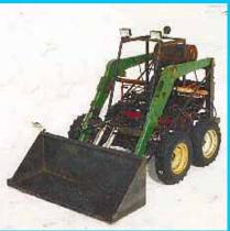
Rob Martens used parts from two swathers to build this skid-steer loader that's powered by a Wisconsin air-cooled engine. He fitted it with lift arms off a Deere front-end loader. (See story on page 2)
