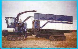
Giant new 20-ton capacity forage harvester was built by custom harvesters in Kansas. It mounts on four hydrostatically-driven sets of rubber tracks, and articulates in the middle. What makes it unique is the rear-mount hopper that eliminates the need to have a truck or wagon alongside. Silage is blown into rear hopper and then unloaded as needed "on-the-go" without ever stopping cutting.
