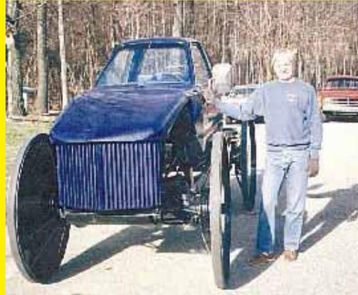
Narrow 2 1/2-in. wide wheels and a cut-down cab make this crop sprayer unique. Larry Hall, Clarkston, Mich., cut 20 in. out of the center of the cab and made a new hood in order to provide enough room for the 4-ft. tall, narrow steel wheels to turn. The narrow wheels let him spray solid-seeded beans without doing damage. See story on page 2.
