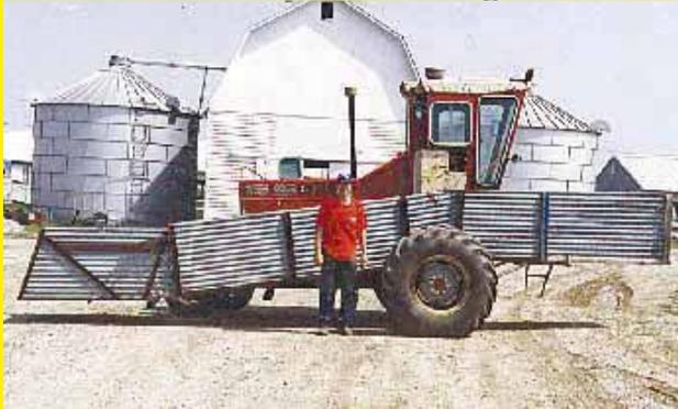
To avoid building a loading chute at each of his eight different finishing buildings, Illinois hog producer Allan Weitkamp built a portable loading chute by mounting a hydraulic-powered chute on the side of his New Idea Uni-Harvester combine. See story on page 2.
