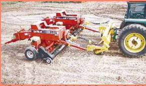
A Texas farmer and his son built a hydraulically powered splitter hitch to pull two Case-IH balers behind their Deere tractor. The hitch also serves as the hydraulic oil reservoir for pumps and motors used to drive the balers.
