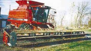
"It's the best down corn harvester ever built," says a Minnesota farmer about his new down corn retriever which lets him recover loose ears and ears still attached to downed stalks. The "Corn Gleener" is built from a 30-ft. Case-IH 1020 grain header and mounts on a "beefed up" Case-IH 2166 combine. See story on page 2.
