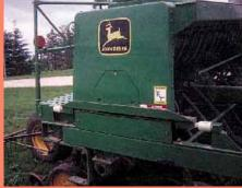
An Iowa farmer mounted electronic weigh scales under each corner of the grain hopper on his Deere 750 grain drill. 'It lets me know how much seed is left in the grain tank at all times and is about 99.5 percent accurate in setting plants per acre,' he says. ''This idea would easily adapt to other makes and models of grain drills.'' Note the white scale units at each lower corner of drill.
