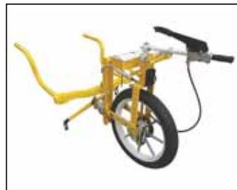
Forecart’s single steering wheel and frame attach directly to any 2-wheeled implement, creating a rigid 3-wheeled unit.
