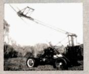
mission ahead of the rear end. I mounted a 1964 Chevrolet engine over the rear end with a three speed hydraulic transmission that drives the four speed through a No. 80 roller chain. I drive the pump off the front of the crankshaft with two V-belts and it works great.
