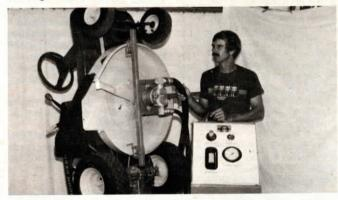
I have been a farm machinery mechanic for the past 17 years. Big dynamometers for large tractors have long been available for in-shop performance tests but when you drop down to lawn and garden tractors there just isn't any way to check performance or load test a mower without finding tall grass. It's tough to adjust a carburetor while bouncing across a lawn.
