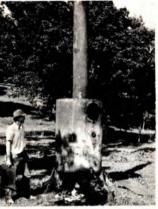
end of the tank, installed a chimney stack on the other end and cut a stoker hole in the side. He sets the stove over the top of a stump and throws in a few wads of paper and some wood to get the stump burning. He says that once you get it burning it keep smoldering until it burns right down below ground to the roots. Key to success of the burner was leaving a gap at the bottom of the stove to provide a steady upward burning draft.
