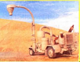
Nebraska farmer mounted an engine and drive axle on a pull-type high-capacity grain vacuum, making a maneuverable rig that gets into tight places a tractor and trailer couldn't go . . . see p. 2.
