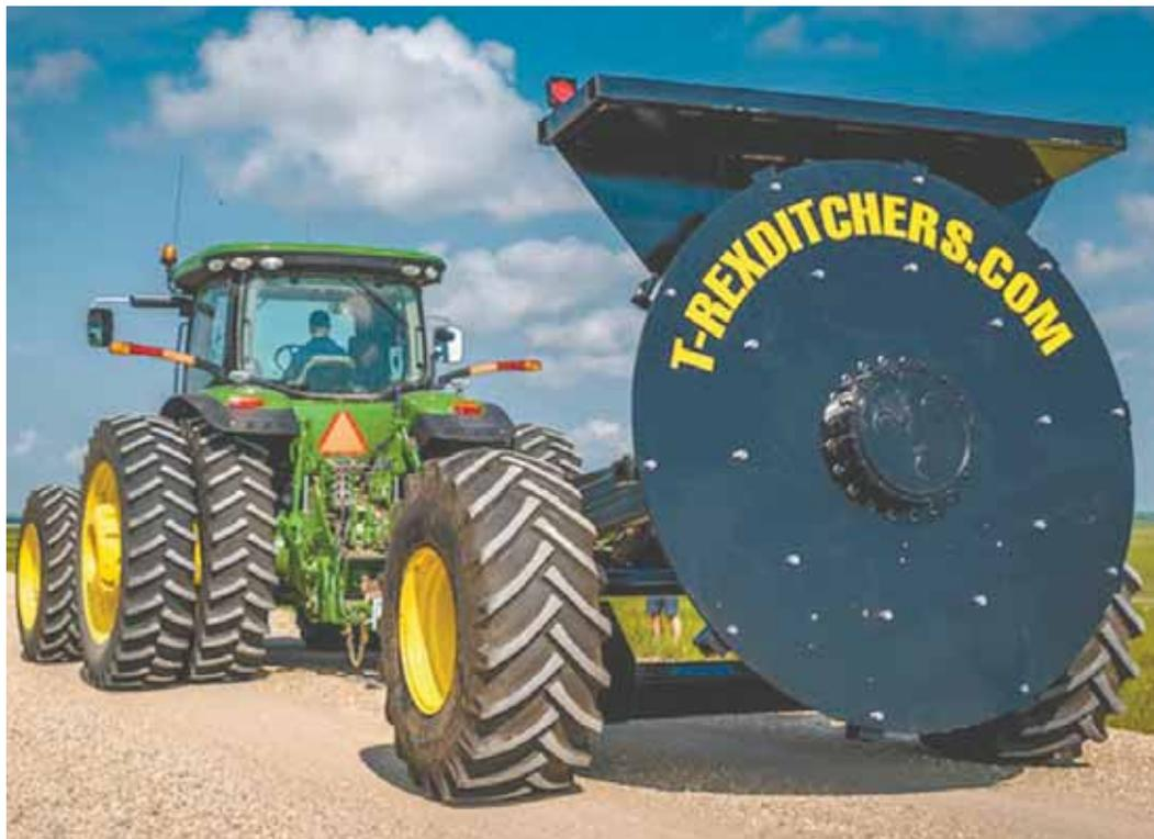
**With its 8-ft. spinning wheel, the T-Rex Rotary Ditcher moves up to 10 times more dirt than pull-type scrapers, backhoes and dozers. And, it throws dirt evenly over a 300-ft. distance without leaving big piles.**
