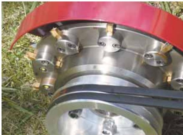
**Stump grinder is powered by a Tecumseh HM80 engine, which double belt-drives the centrifugal clutch to the grinder's teeth.**
