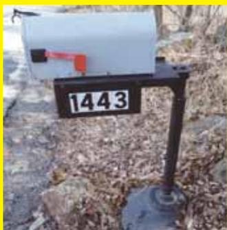
In the past few years, my mailbox was destroyed 3 times by snowplows. I decided to build a swing-away mailbox by using the cast wheel and axle from a Farmall A. I slipped a long piece of pipe over the axle and then inserted a
