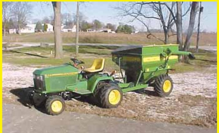
I built a grain cart to pull behind a John Deere garden tractor that has a 540 pto to operate the grain auger. The grain gate on the auger opens and closes by hydraulics and the auger also folds up and down with a hydraulic cylinder. It also has a hand-rolling tarp. I also put dual wheels on the garden tractor.
