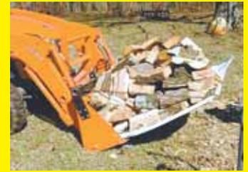
I made this bucket extender for my front-end loader from a scrap car hood and some old chains. The hood slips into the loader bucket and a chain runs from the top of the bucket to the outer corner of each side of the hood. It's great for carrying wood and other bulky loads. **(Frank Heraghty, Claremore, Okla. (ph 918 342-5809)**
