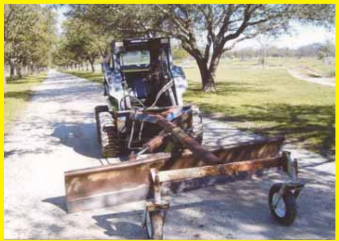
Here's a photo of a skid loader-mounted road grader that I built out of scrap materials.
