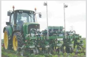
"Robo Weeder" is guided by 2 video cameras that use color and pattern recognition software to identify weeds, then synchronize that information with weeding discs.
