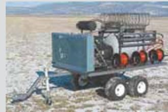
**Pressurized Exhaust Rodent Control machine forces pressurized carbon monoxide into tunnels to kill gophers.**
