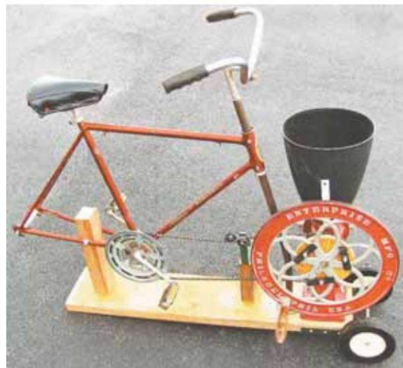
By converting his antique, hand-operated shelled corn grinder to pedal power, Philip Whitmoyer made grinding small batches of corn a much easier job.
