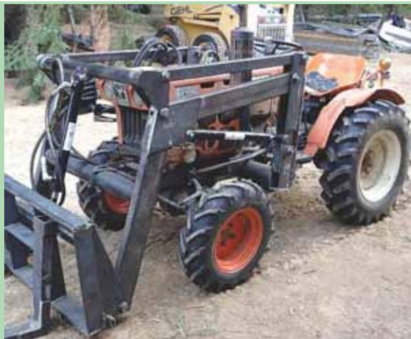
Kevin Ranette can custom-build front-end loaders for almost any tractor, big or small. Standard features include mechanical self-leveling and quick-tach loader frame.
