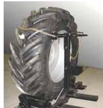
**Wheel EZ tire changer comes with a pair of welded-on metal tubes so pallet forks can pick it up. It's built with 2 telescoping halves fitted on each side with 3 metal rollers that support tire.**
