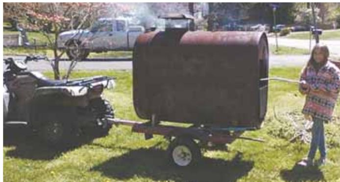
**Burn barrel is built out of a 275-gal. fuel tank and mounted on a 2-wheeled trailer. "It's much safer than burning debris out in the open on the ground," says inventor John Jett.**
