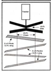
I've used this system for 30 years to prepare fields. I bolt 4 planks to a pair of chains behind a disk. The planks are positioned at an angle. They level the field and are easy to pull yet they won't plug. I use one 2 by 6 plank 12 ft. long and three 2 by 4's 14-ft. long behind my 10-ft. disk. (Ernest Ivany, Box 533, Lister, B.C. VOB1Y0)
