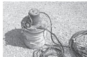
electric motor mounted on top of the cover plate. The motor drives a shaft that goes down inside the bucket and is connected to a small can and pump, which pumps the grease out.
