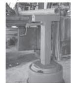
needed, depending on what you're cutting. I made it from an old trailer jack. I first cut it down to the right length, and then welded it to a used 20-in. truck rim. A 16-in. roller attaches to the top. With a turn of the crank. a full load of materials can be adjusted to the desired height. Very handy."
