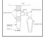
Edwards' design involves removing the sediment bulb from bottom of fuel tank and putting a "trap" for larger sediment in its place.
