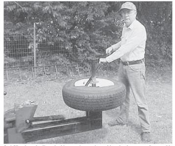
Jack Vines' wood splitter doubles as a tire repair machine, thanks to a set of removable attachments.
