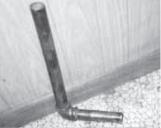
I made one using his directions and it's the handiest fencing tool I have. It's made from two 1-in. pieces of pipe connected by a 90 degree elbow. The handle, is 16 in. long and the other is 8 in. long. A 5/16-in. dia. hole is drilled through the 8-in. piece, 2 in. out from the elbow.
