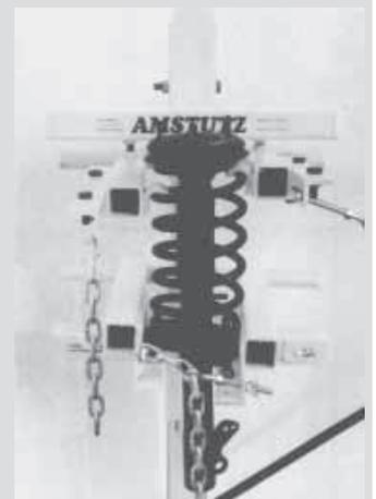
Hydraulic coil spring compressor can be used to remove damaged coil springs from most cars and pickups, as well as ATV's and other equipment.
