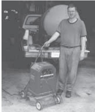
**Dennis and Roger Koelling, Bartelso, Ill.:** "By mounting our Lincoln AC-DC electric welder on the deck of an old 22-in. push mower, we can easily move the welder anywhere inside our shop."
