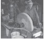
Noel Hicks, Palmyra, Ill.: He took an old foot-powered grindstone, built a stand for it and motorized the grindstone. It works a lot better than modern high-speed grinders because it grinds slowly and doesn't burn the edges as fast, says Hicks.
