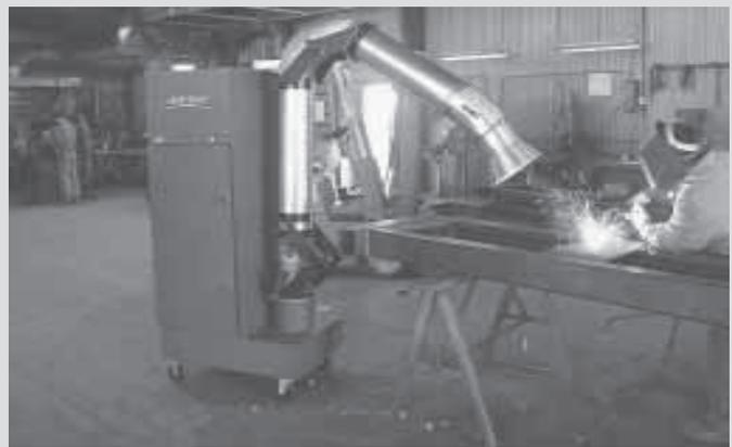
Air cleaner rides on four caster wheels. Suction arm on front draws dirty air into the unit before it has a chance to get out into shop.
