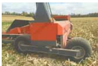
Harvester frame mounts on a long oscillating tandem axle mounted under the impeller. Kernels and cobs are crushed fine before being blown into wagon.
