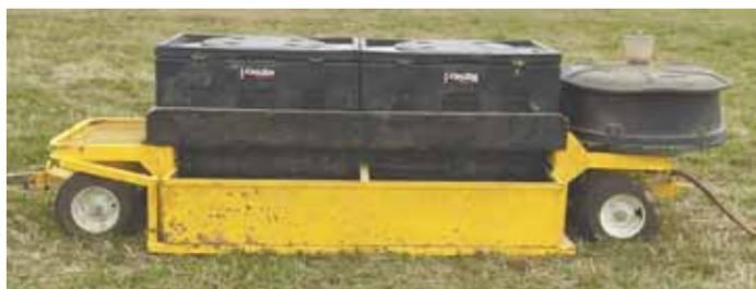
Doug Abney's rotational grazing system includes this combination watering system/mineral trailer/tool cart that rides on a 4 by 10-ft. trailer.
