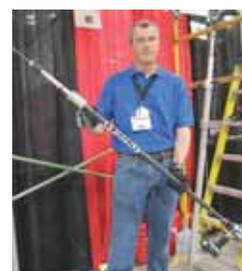
Cordless drill attaches to lower end of Kwik Pole for overhead drilling.
