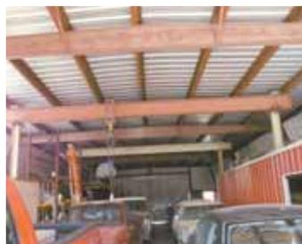
Overhead shop hoist moves back and forth on a 24-ft. long I-beam supported at each end by a vertical steel beam.
