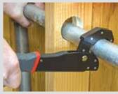
The self-adjusting head instantly grabs and releases pipes. You position the wrench around the material, then press the head forward or pull up on the jaw to release and re-engage.
