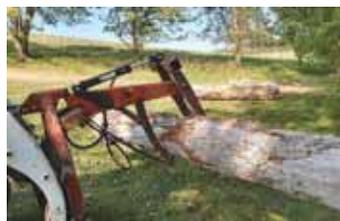
Grapple uses a pair of 3-ft. long curved, movable jaws spaced 12 in. apart, and 2 fixed shanks.
