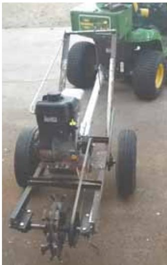
When Thomas Schraufnagel built this towable stump grinder, he designed the frame and pulley drive so it could do double duty as a tiller.
