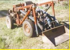
Bob Burk of Hutchinson, Kan., built an articulated, mini-4-WD tractor that does the work of a skid steer. Burk used a pair of auto axles cut down to 3 ft. wide. See story on page 2. Ray Skoglund decided to build this skid-steer after reading about a similar home-built rig in FARM SHOW. He used parts from two self-propelled swathers. See story on page 2.
