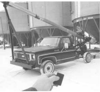
Wahouske mounted the 40-ft. long, 8-in. dia. auger on a 1974 Chevy pickup. He uses four car door lock actuators to turn the auger on and off from up to 75 ft. away.
