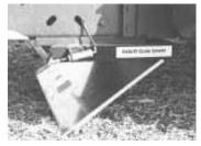
An air cylinder drops the pan while the combine is moving through the field.
